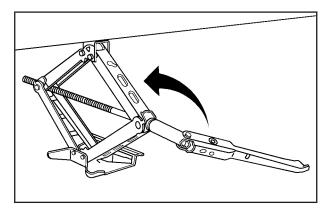
13. Lower the vehicle by attaching the wheel wrench to the jack and turning the wrench counterclockwise. Lower the jack completely.
